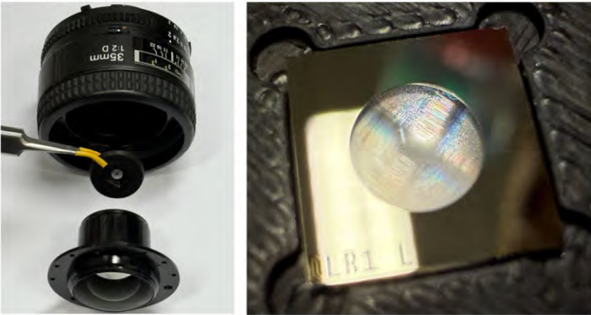
Learned Diffractive Optical Element (DOE)
